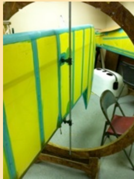
A wing mounted in a rotisserie jig at our Clubhouse.
