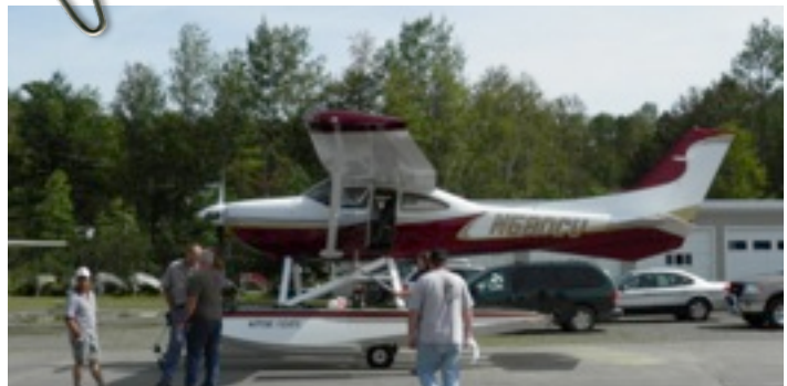
Above: Experimental C-182 with new floats, 580 cu.in. on the firewall with an MT prop. Below: A beautiful day on Moosehead Lake, as the Katahdin departs from Greenville, Maine.
