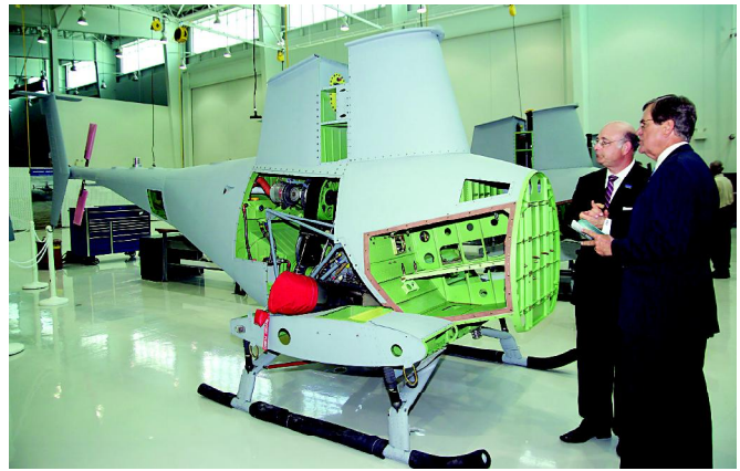
Composite materials are used to assemble UAVs such as the Global Hawk aircraft (left) and the Fire Scout helicopter (right). Photos courtesy Northrop Grumman Corp.
