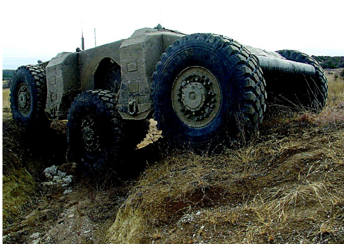
This 6.5-ton unmanned military vehicle uses six electric motors embedded in each wheel. Photo courtesy Carnegie Mellon University
