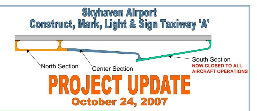
The work on the South Section of Taxiway 'A' started as scheduled on October 23<sup>rd</sup> with all pavement reclamation now completed. Grading and base material will be placed on the South Section of Taxiway 'A' starting October 25<sup>th</sup>. Paving is anticipated to start on Wednesday, October 31<sup>st</sup>, weather permitting. The FBO maintenance hangar will be accessible on a prior notice required basis.
