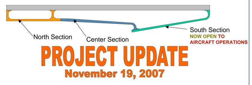
The construction work to the south section of Taxiway 'A' was substantially completed today, November 19, 2007. In the spring, after the snowplowing season, the contractor will return to this section of pavement to place the 2<sup>nd</sup> coat of taxiway paint markings, relocate the easterly edge of taxiway lights, and hydroseed the easterly taxiway shoulder. In the meantime, the project area will be stabilized for the winter and cleanup activities will be wrapping up shortly.
